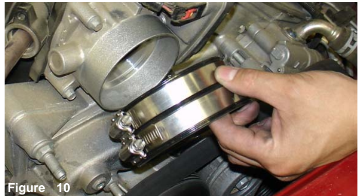
Figure 8 Once the fuel pressure regulator line and the bolt on the air box have been removed continue to pull the entire air intake assembly as shown above.
