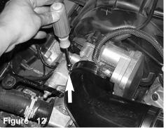
Once you have adjusted the elbow over the throttle body continue to simi-tighten the clamp.
