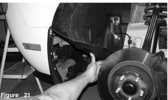
The mudd flap will be pulled back when your ready to install the filter.
