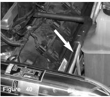
Be sure to insert hose  $3\!/\!4"$  over the intake port for firm grip.
