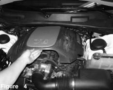
The engine cover stand-offs are pulled up and out of grommets, now your ready to remove the cover from the engine compartment.
