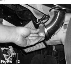
The filter clamp is tightened once the filter has been properly positioned.
