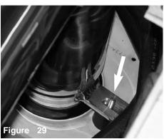
The intake bracket is sitting flush over the vibra-mount stud.
