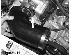
Place clamps over ecah end of the 3 1/2" elbow, slip elbow over the end of the throttle body as shown above.
