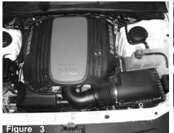
Stock air intake box and air intake duct shown above.
