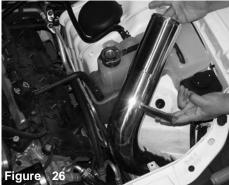
The intake is slowiy rotated in clockwise position while lowering it into the resonator opening.
