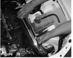
The intake is placed into the engine compartment with the long side facing the firewall. The filter end is slowly inserted into the resonator opening.
