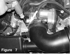
Loosen the clamp located over the throttle body. This will be necessary in order to remove the air duct.
