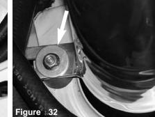
The m6 flange nut is tightened over the washer as shown above.
