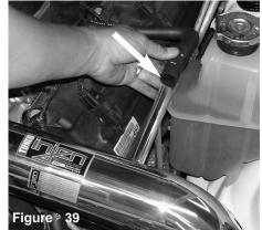
The stock crankcase hose is pressed over the intake port.
