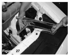
The intake is lowered in position while the intake bracket is aligned to the vibra-mount stud.
