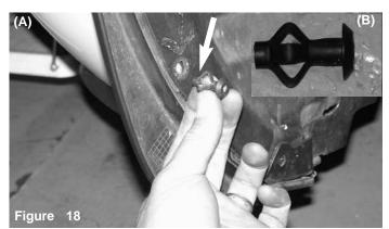
The plugs are now removed (A). The plug pulled out is shown above (B).
