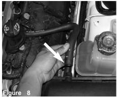
The crank case hose is pulled off the air box port as shown above.
