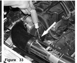
The clamp over the intake is now tightened.
