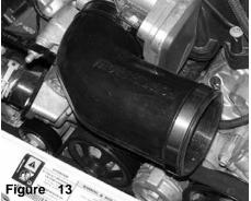
The 3  $/2^{\prime\prime}$  elbow is now installed over the throttle body and ready for the next step.
