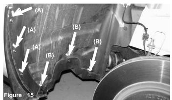
Once you have removed the tire you will be removing three side bolts and plugs (A), and three lower plastic pins (B). Removal of all plastic clips will allow you to pull the mudd guard back to install the filter.
