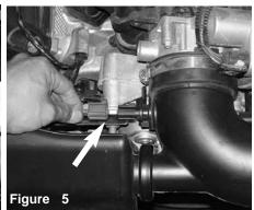
The electirical harness clip is pulled from the air temperature sensor. The tab on the clip is pressed down before you pull the clip from the air sensor.
