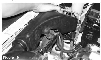
Prior to pulling the air box and air duct from the engine compartment, pull up on the resonator box located on the passenger side. Once you have dislodged the resonator box continue to up the air box cleaner out of the engine compartment.
