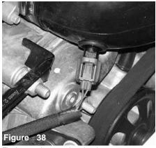
The harness is pressed on the air temperature sensor until it snaps in place.
