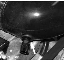
The air temperature sensor is installed in the grommet.
