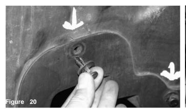
All three lower clips are now removed along with the pins.
