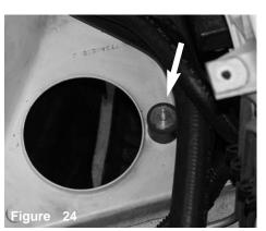
The vibra-mount is now installed in place.
