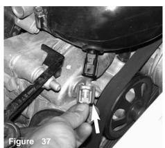
The electrical sensor harness is aligned to the air temperature sensor.
