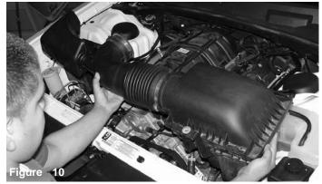
Once all clamps and bolts have been loosened or removed, continue to pull the entire air box cleaner from the engine compartment.
