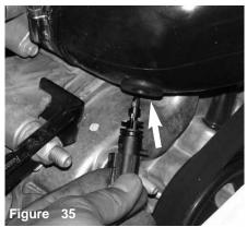
The air temperature sensor is lined up to the grommet and pressed in until it sits flush over the grommet.
