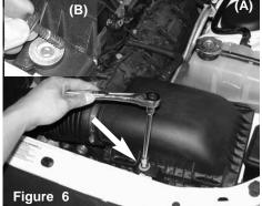
Loosen the m6 bolt located in front of the air box (A) once you have loosened the bolt, continue to remove the bolt (B).
