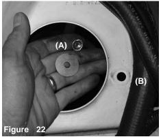
The m6 flange nut and washer are held under the resonator opening (A) as the vibra-mount is lowered into the small hole(B).
