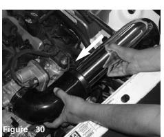
The intake is slowely pressed into the 3 1/2" elbow as shown above.
