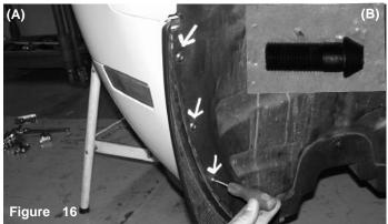
A screwdriver is used to remove all three screws before pulling the plug the out (A). A screw is pulled out of the plug after it is loosened (B).
