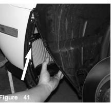
The mudd guard is pulled back and the filter is aligned to the end of the intake.
