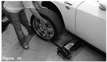
In order to install the cold air intake, it will be necessary to lift the front drivers of the car. Once you have lifted the car, continue to removed the front, driver side wheel.
