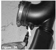
The air temperature is removed from the stock air intake duct.
