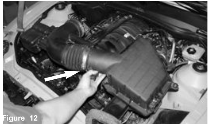
Figure 11 Remove the two m6 nuts holding the air box cleaner to the strut tower mount.
