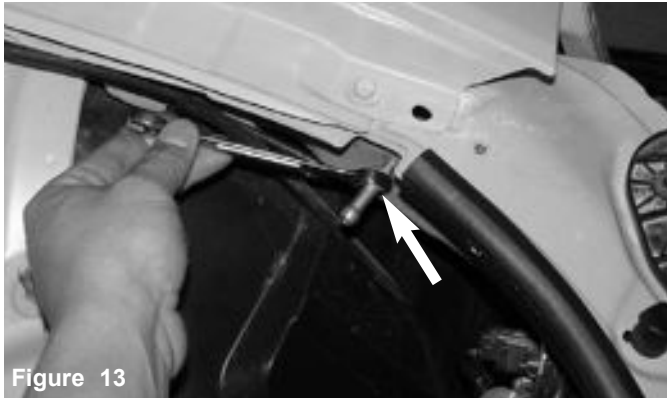
Figure 11 Remove the two m6 nuts holding the air box cleaner to the strut tower mount.
