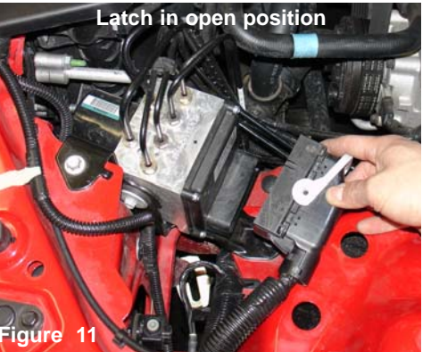
Figure 11 The latch is in the open position and the harness clip is removed from the ABS solenoid.
