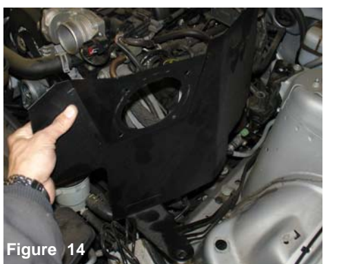
Figure 14 The heat shield is now lowered into the engine compartment and the top bracket is aligned to the strut tower mount and the lower bracket is aligned to the ABS solenoid.
