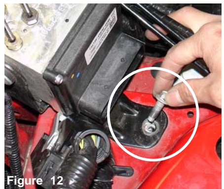
Figure 12 Remove the m6 bolt that fastens the ABS solenoid leg to the car frame.
