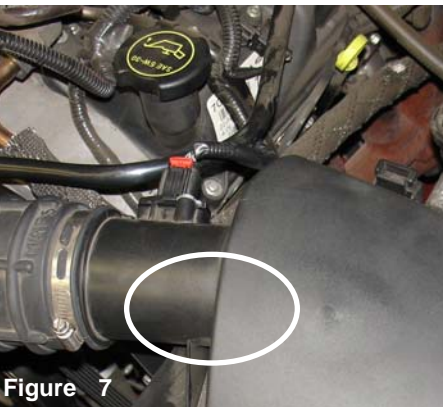
Figure 7 The bolt holding the air box bracket is loosened and removed. This will allow the air box to be pulled out of the engine compartment.
