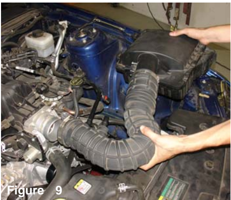
Figure 9 Remove the entire air intake duct and air intake cleaner from the engine compartment.
