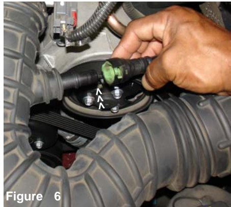
Figure 6 The crank case hard pipe breather line is disconnected.
