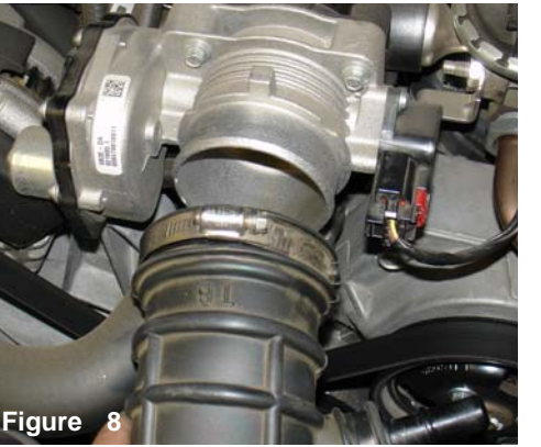
Figure 8 Once the clamp has been loosened continue to remove the air duct from the throttle body.
