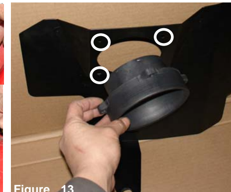
Figure 13 The bolt pattern on the composite velocity stack is aligned to the heat shield bolt holes.
