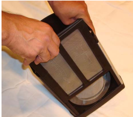
The rectangular pre-filter screen is now slipped out of the channel along the body of the power box.
