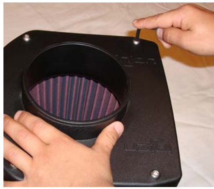
Unbolt the four- m6 x 20mm screws from the velocity stack base located to the center of the base. Now separate the base from the velocity stack.
