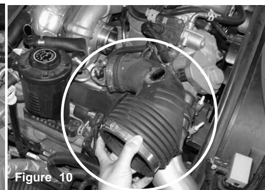
Figure 10 You may now pull the intake turbo air duct out of the engine bay.
