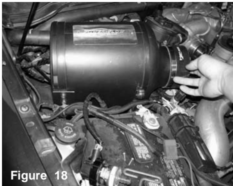
Figure 18 Position the Injen air box assemble into the factory air box location.
