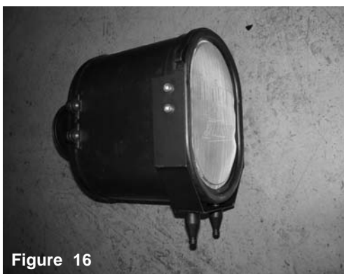
Figure 16 Air box and bracket completely assembled
