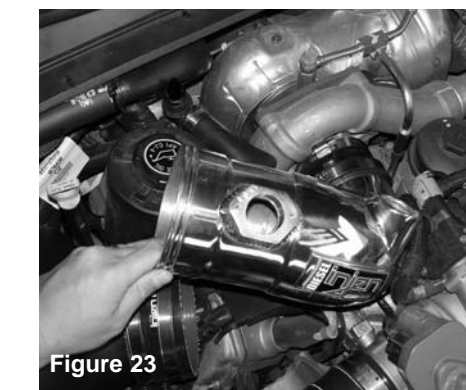
Figure 23 Slip the step hose end of the cast intake over the centering spacer previously installed on the turbo inlet in figure 21.
