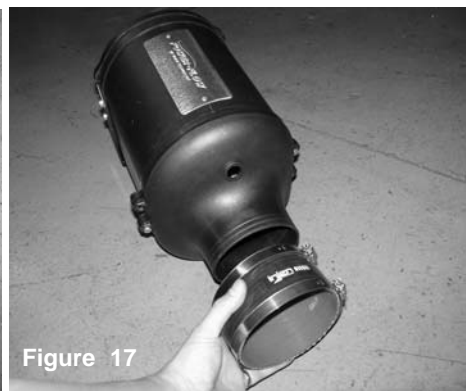
Figure 17 Place the 4 5/8" straight hose onto the outlet of the air box assembly and only tighten the clamp on the air box side.
