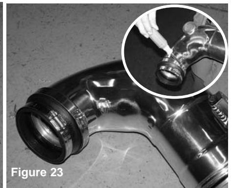
Figure 23 Step hose shown mounted on the cast intake. Now tighten the clamp on the cast intake side as shown in the photo.
