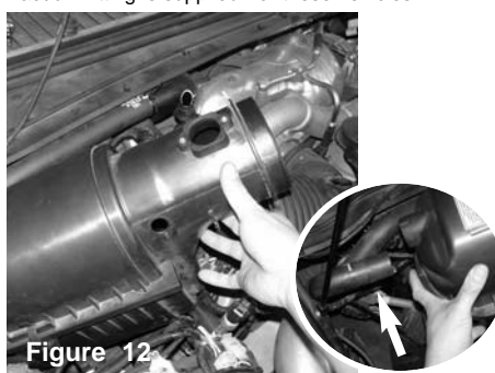
Figure 12 Firmly lift up on the air box assembly and remove the air box from the engine bay. Make sure you remove the auxiliary heat tube from the air box
