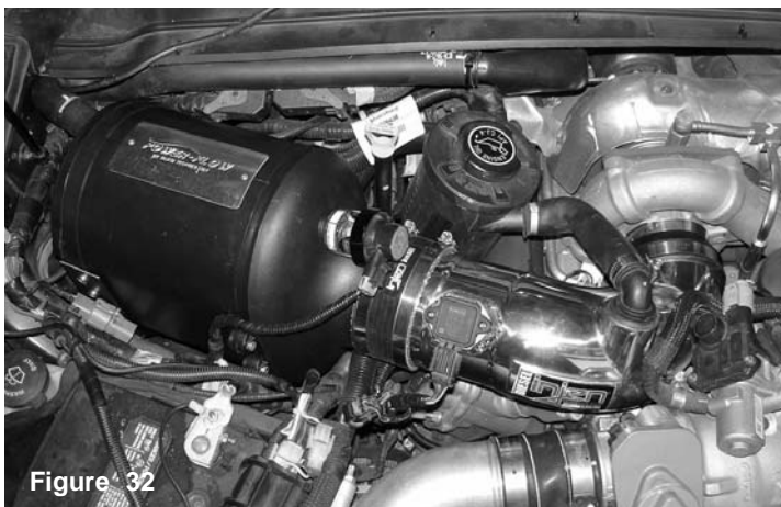
Figure 32 Check the entire system for the best possible fit. Once you have checked the entire system for leaks, rubbing or rattling, continue to tighten all nuts, bolts and clamps. Reconnect the negative battery terminal prior to starting the engine.
