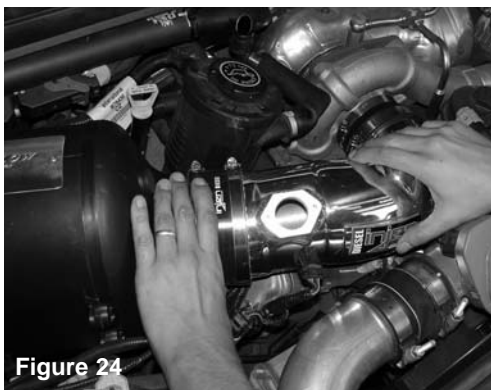
Figure 24 Now connect the other end of the intake tube into the 4 5/8" straight hose on the Injen air box
