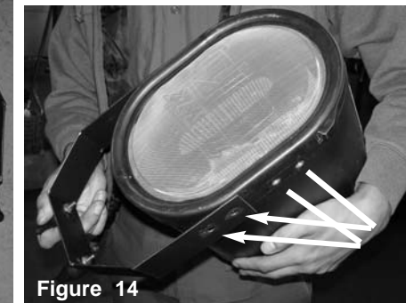
Figure 14 Position the air box bracket and align the two 3/8" holes on each side of the bracket onto the two threaded inserts on each side of the air box
