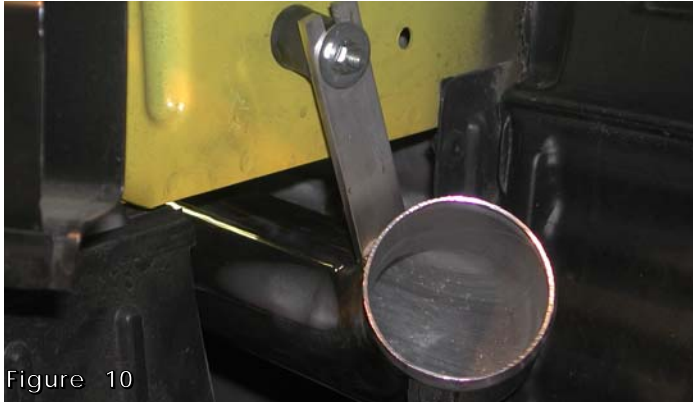
Figure 10 Line up the bracket on the end of the secondary intake to the vibra-mount stud. Use the m6 flange nut and bolt to secure the intake to the vibra-mount.
