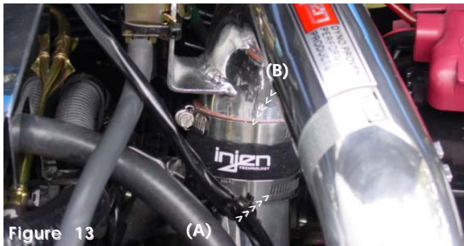
Figure 13 Once the 2 1/4" tapered side of the intake has been inserted into the hose on the throttle body, press the top end(B) into the hose on the end of the secondary intake(A). (A) seen here is the end of the secondary intake and (B) is the end of the primary intake.
