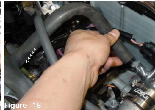
Figure 18 Take the other end of the 15mm hose and press it over the end of the 5/8" port on the intake, again use the stock clamp.
