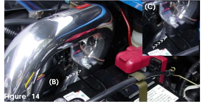
Figure 14 The primary intake is now line up the bracket to the vibra-mount stud(B). Use the m6 flange nut and fender washer to hold the intake in place(C).
