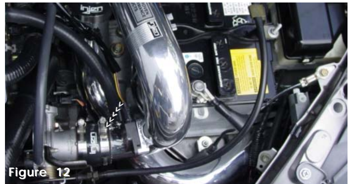
Figure 12 The primary intake is lowered into engine compartment. The end with the 2 1/4" diameter is pressed into the hose on the throttle body. The clamp is then semi-tightened on the intake to hold it in place.
