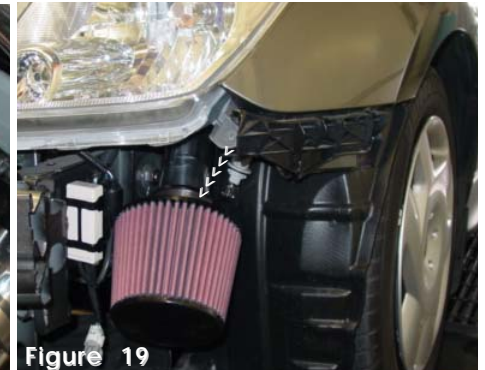
Figure 19 Before the cold air intake is aligned and bolted in place press the filter over the end of the secondary intake and fasten the clamp on the filter neck.
