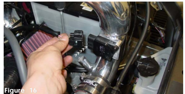
Figure 16 Press the harness clip into the air flow sensor on the machined adapter. You will hear a snapping sound when the harness and sensor are properly attached.
