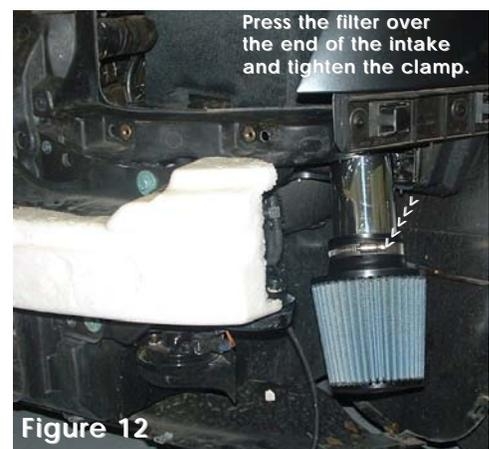
**Note: Disconnect the negative battery terminal before starting this installation.**
