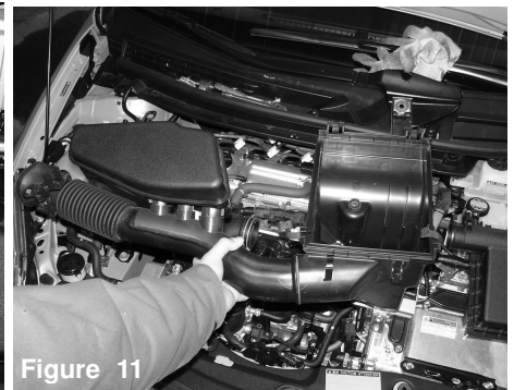
Figure 11 you may now remove the entire lower portion of the airbox cleaner.
