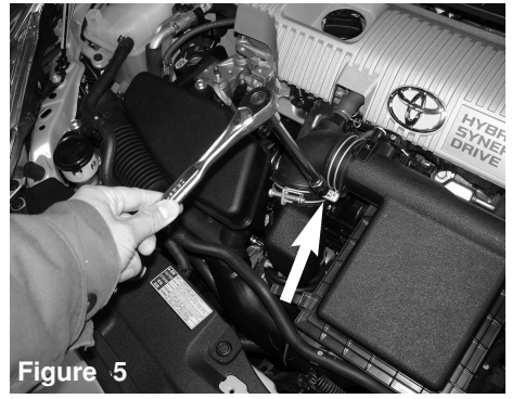
Figure 5 Loosen clamp from throttlebody air duct to air box cleaner using a 10mm socket and 3/8 ratchet
