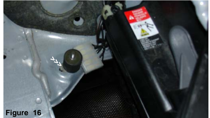
Figure 14 Remove the bolt that grounds the wire connectors to the frame. This is where the vibra-mount will be placed.
