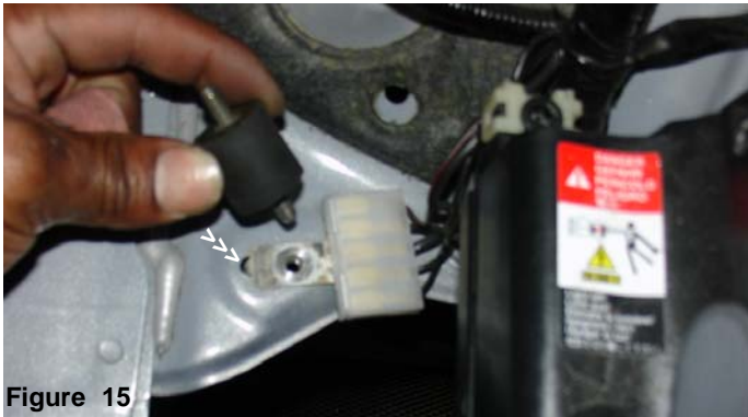
Figure 16 The vibra-mount is screwed in place until it sits flush over the connector plate.
