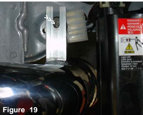
Figure 17 Lower the intake into the engine compartment, align the top end to the inlet hose and the intake bracket to the vibra-mount stud.
